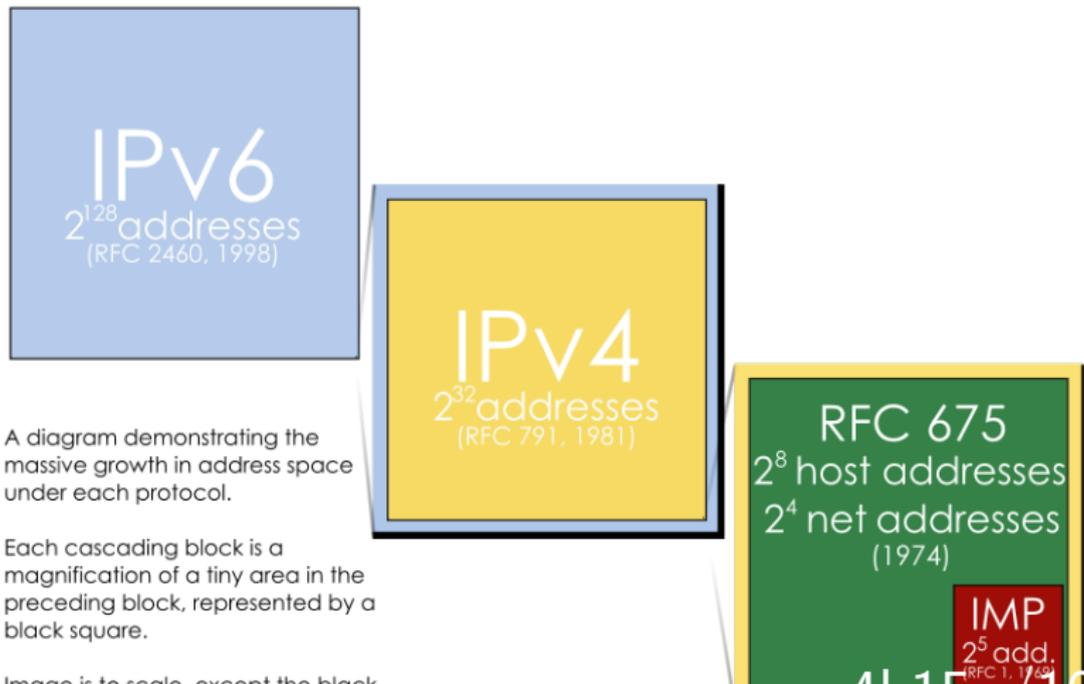
A diagram demonstrating the massive growth in address space under each protocol.
